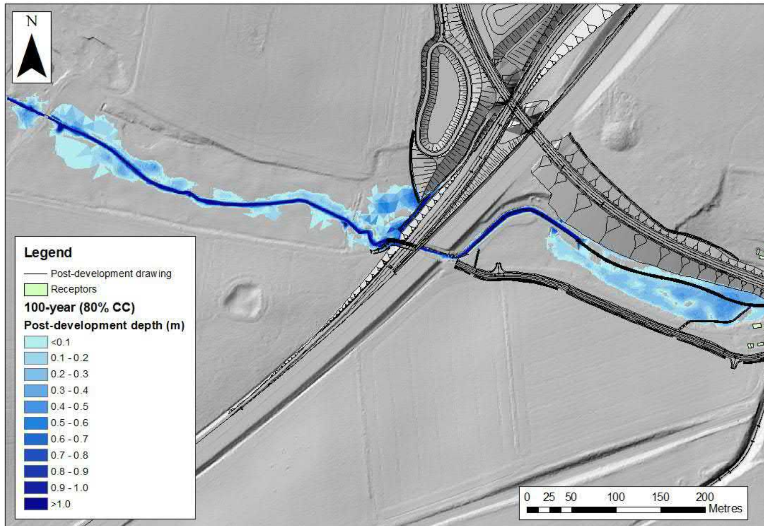
Figure C.4 : Maximum post development flood depths between upstream boundary and Cantley Lane South (100-year event with 80% climate change)
