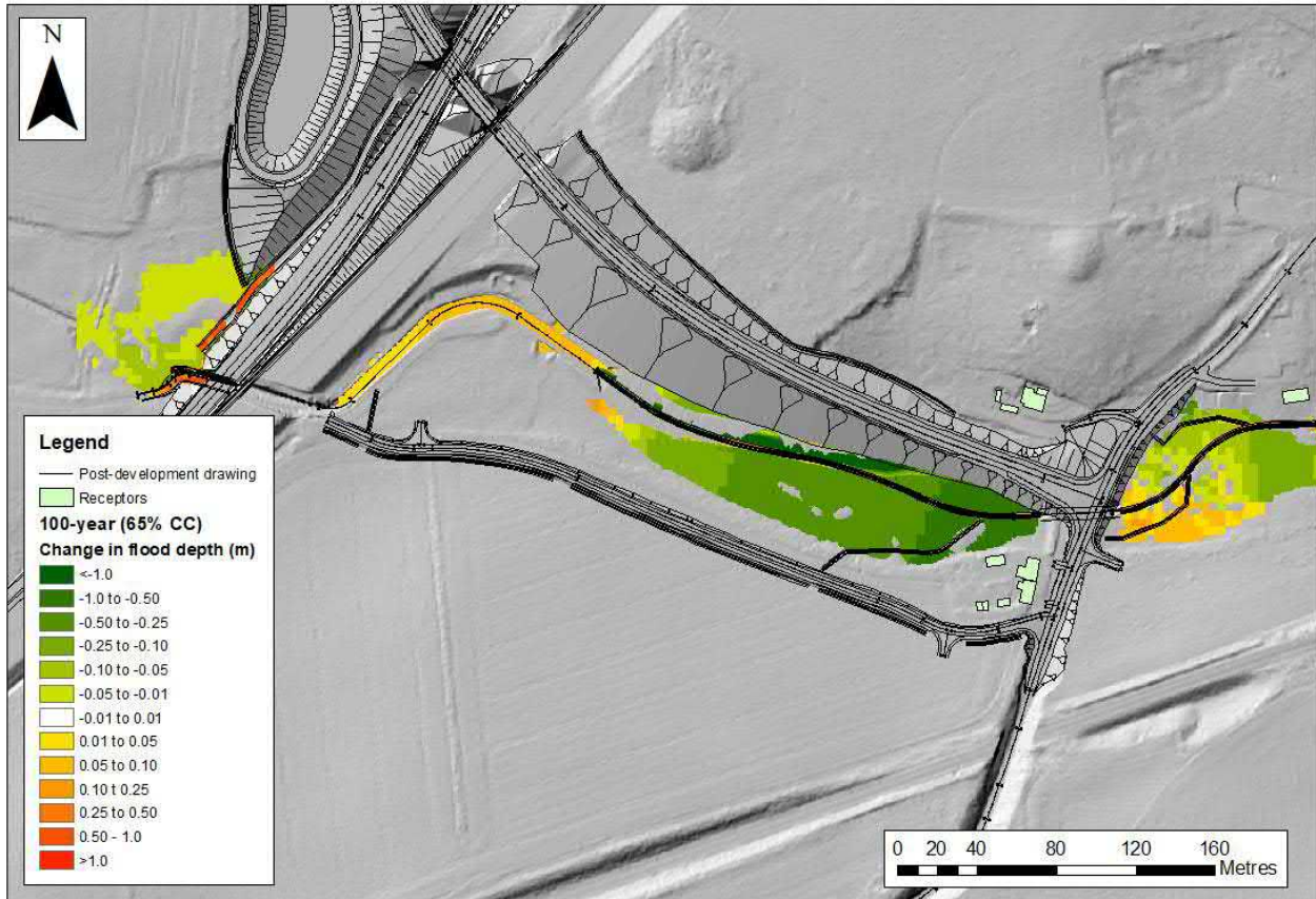
Figure 8-4: Flood depth difference for the 100-year plus 65% climate change event between the baseline and post-development modelling of the realigned Cantley Stream
