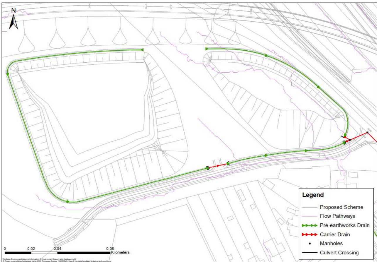
Figure 8-10: Proposed earth bund drainage arrangements
