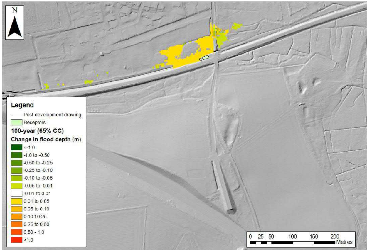
Figure 8-6: Flood depth difference for the 100-year plus 65% climate change event between the baseline and post-development model between A47
