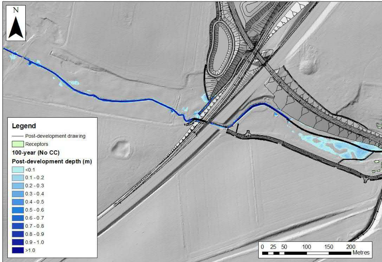
Figure C.1 : Maximum post development flood depths between upstream boundary and Cantley Lane South (100-year event with no climate change)
