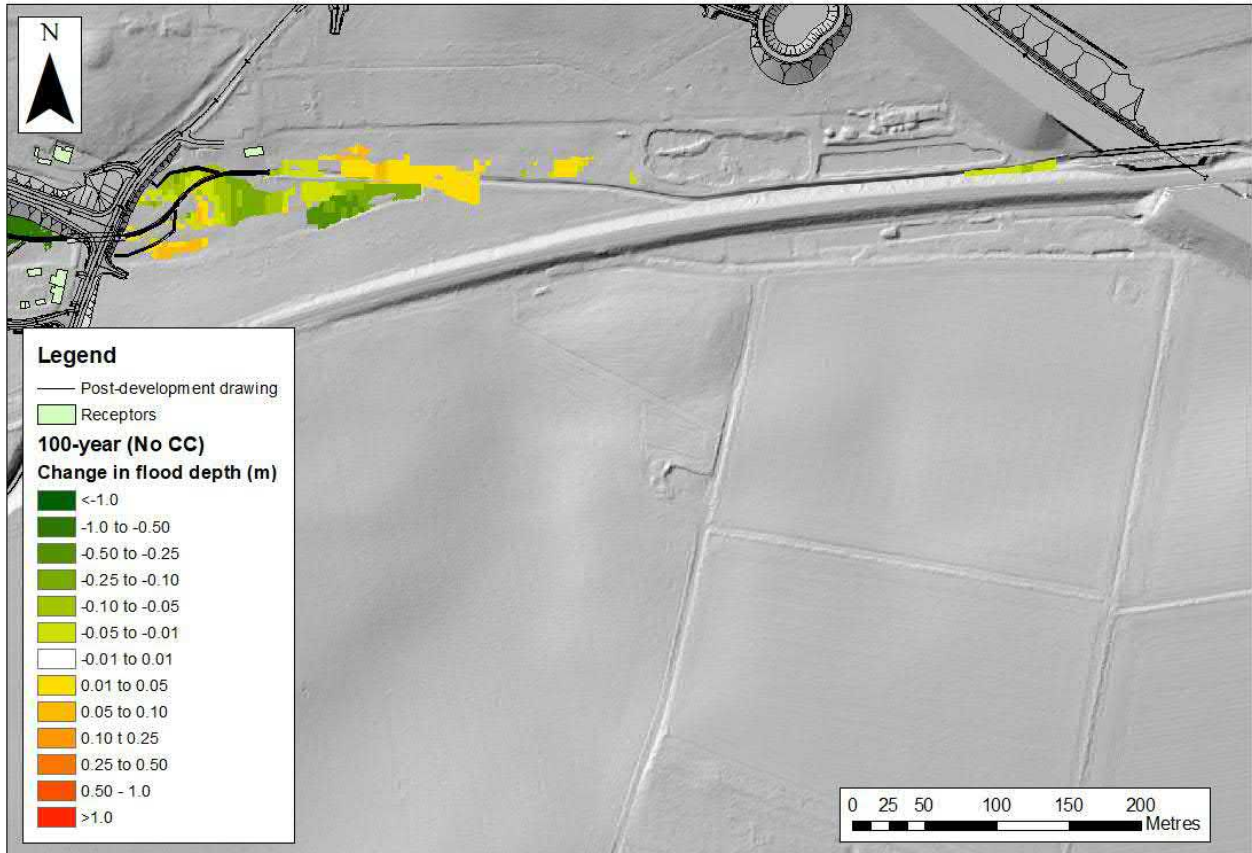
Figure 8-2: Flood depth difference for the 100-year event between the baseline and post-development model between Cantley Lane South culvert and A47
