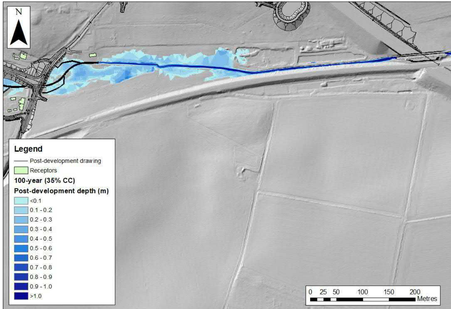
Figure C.7 : Maximum post development flood depths between Cantley Lane South and the A47 (100-year event with 35% climate change)
