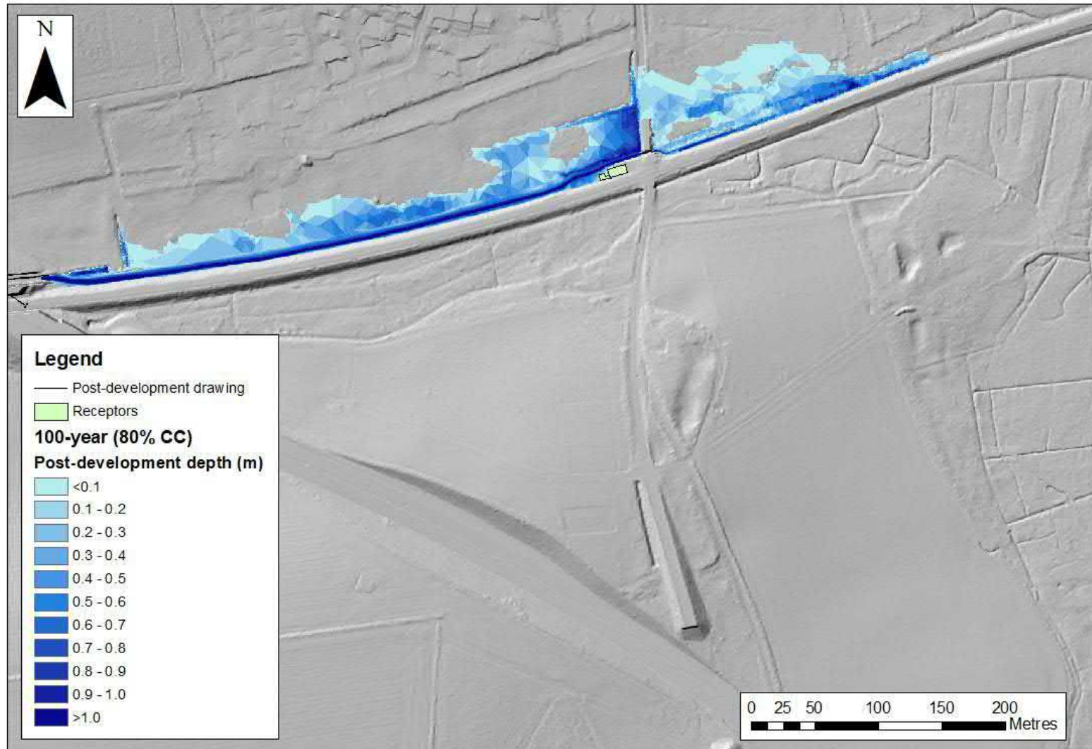
Figure C.14 : Maximum post development flood depths between the A47 and the model outfall (100-year event with 80% climate change)
