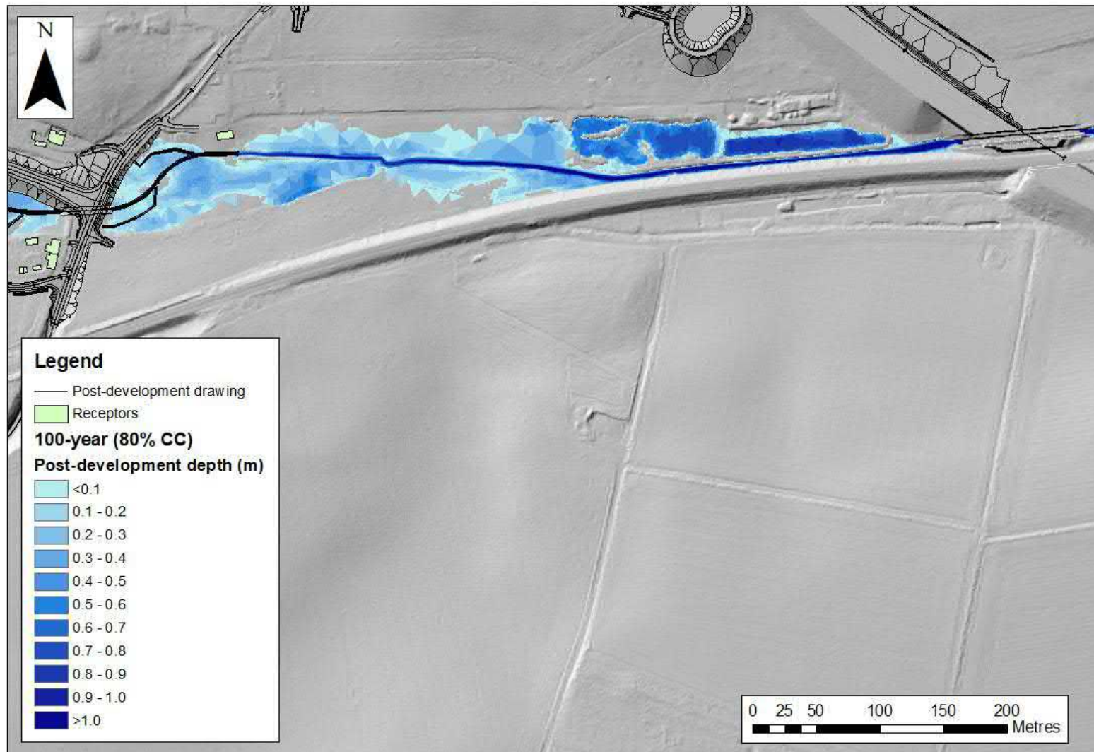
Figure C.9 : Maximum post development flood depths between Cantley Lane South and the A47 (100-year event with 80% climate change)
