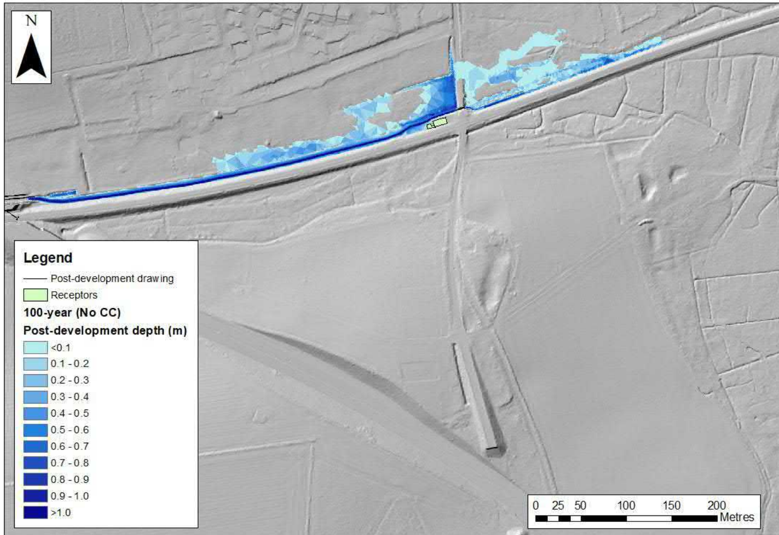
Figure C.11 : Maximum post development flood depths between the A47 and the model outfall (100-year event with no climate change)
