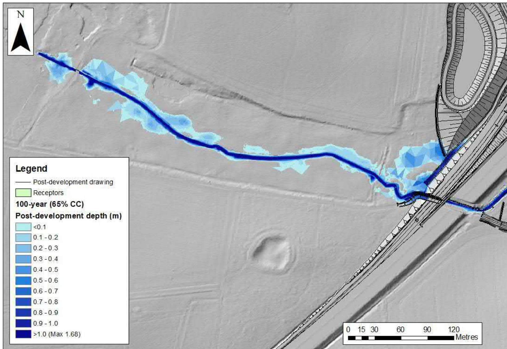
Figure A.4 Maximum predicted depths between upstream boundary and A11 for post-development scenario
