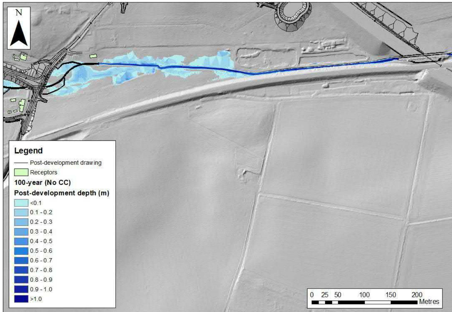
Figure C.6 : Maximum post development flood depths between Cantley Lane South and the A47 (100-year event with no climate change)
