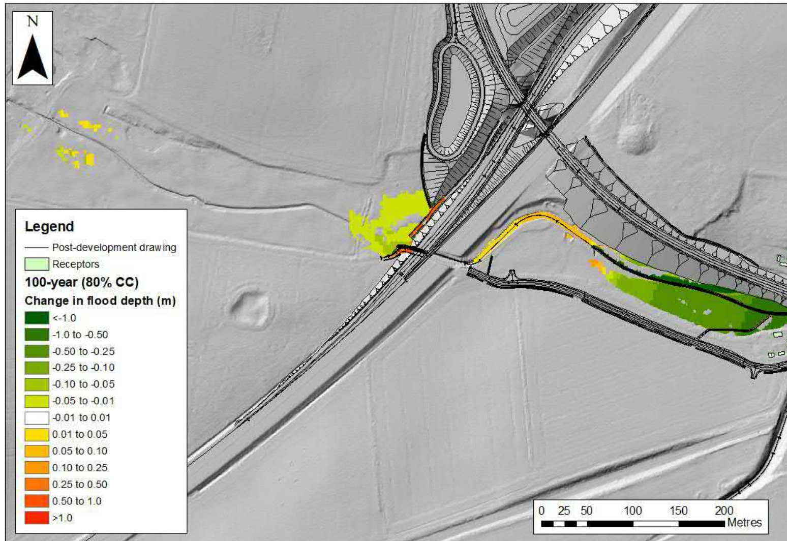
Figure C-4: Flood depth difference between upstream boundary and Cantley Lane South (100-year plus 80% event)
