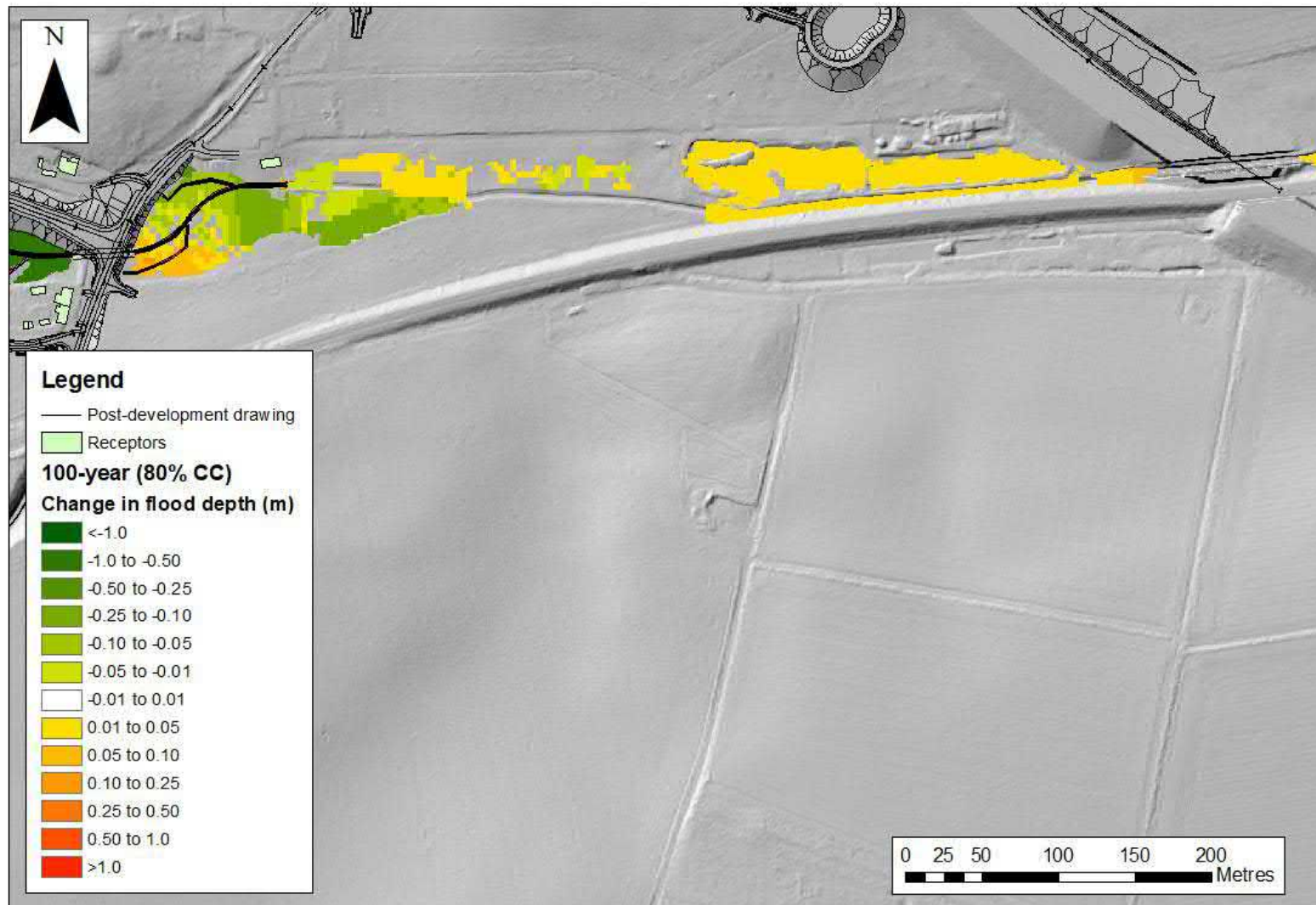
Figure C-9: Flood depth difference between Cantley Lane South and A47 (100-year plus 80% event)
