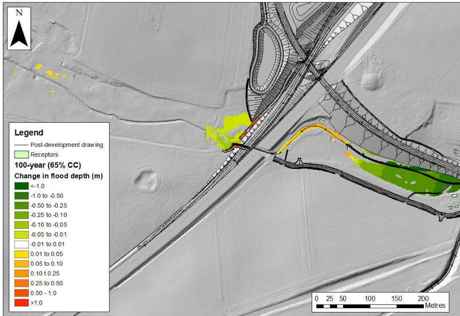
Figure C-3: Flood depth difference between upstream boundary and Cantley Lane South (100-year plus 65% event)
