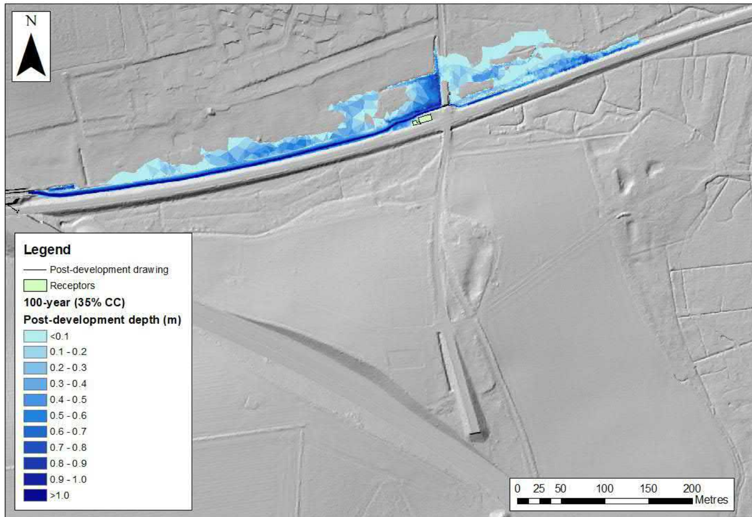
Figure C.12 : Maximum post development flood depths between the A47 and the model outfall (100-year event with 35% climate change)
