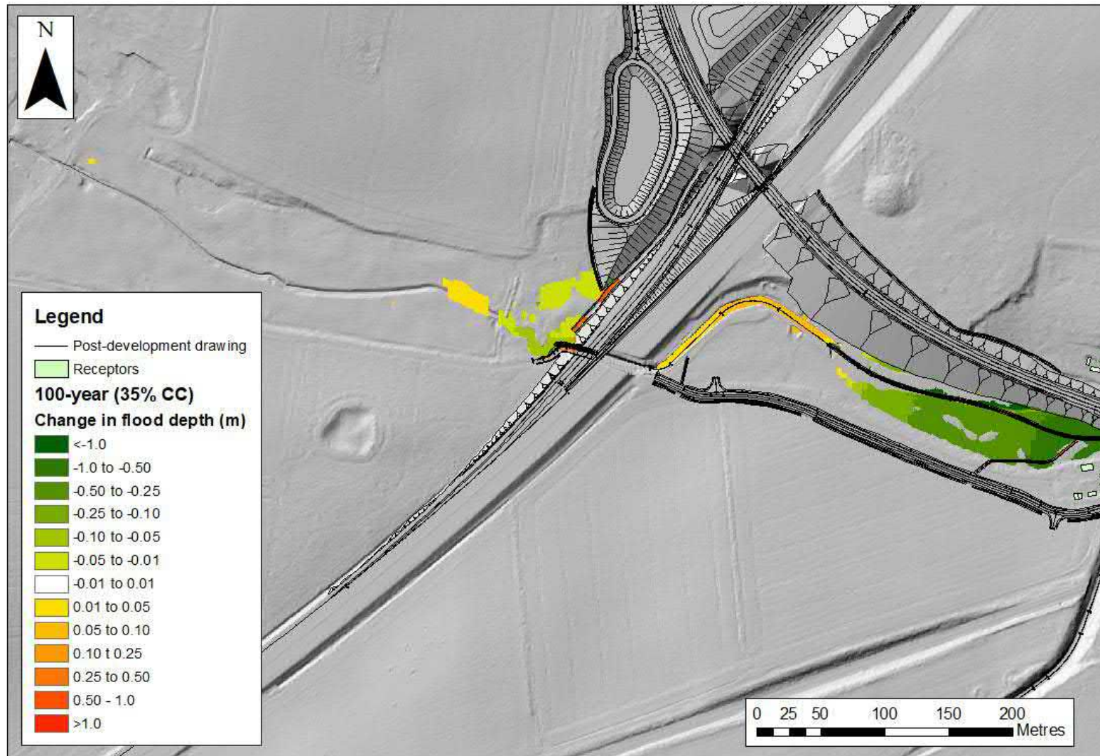
Figure C-2: Flood depth difference between upstream boundary and Cantley Lane South (100-year plus 35% event)
