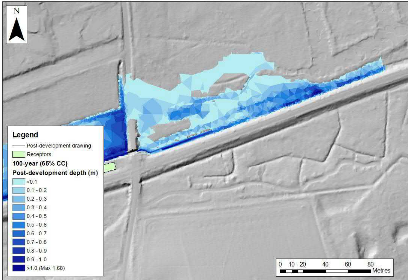
Figure A.16 Maximum predicted depths between Intwood Road and downstream boundary for post-development scenario
