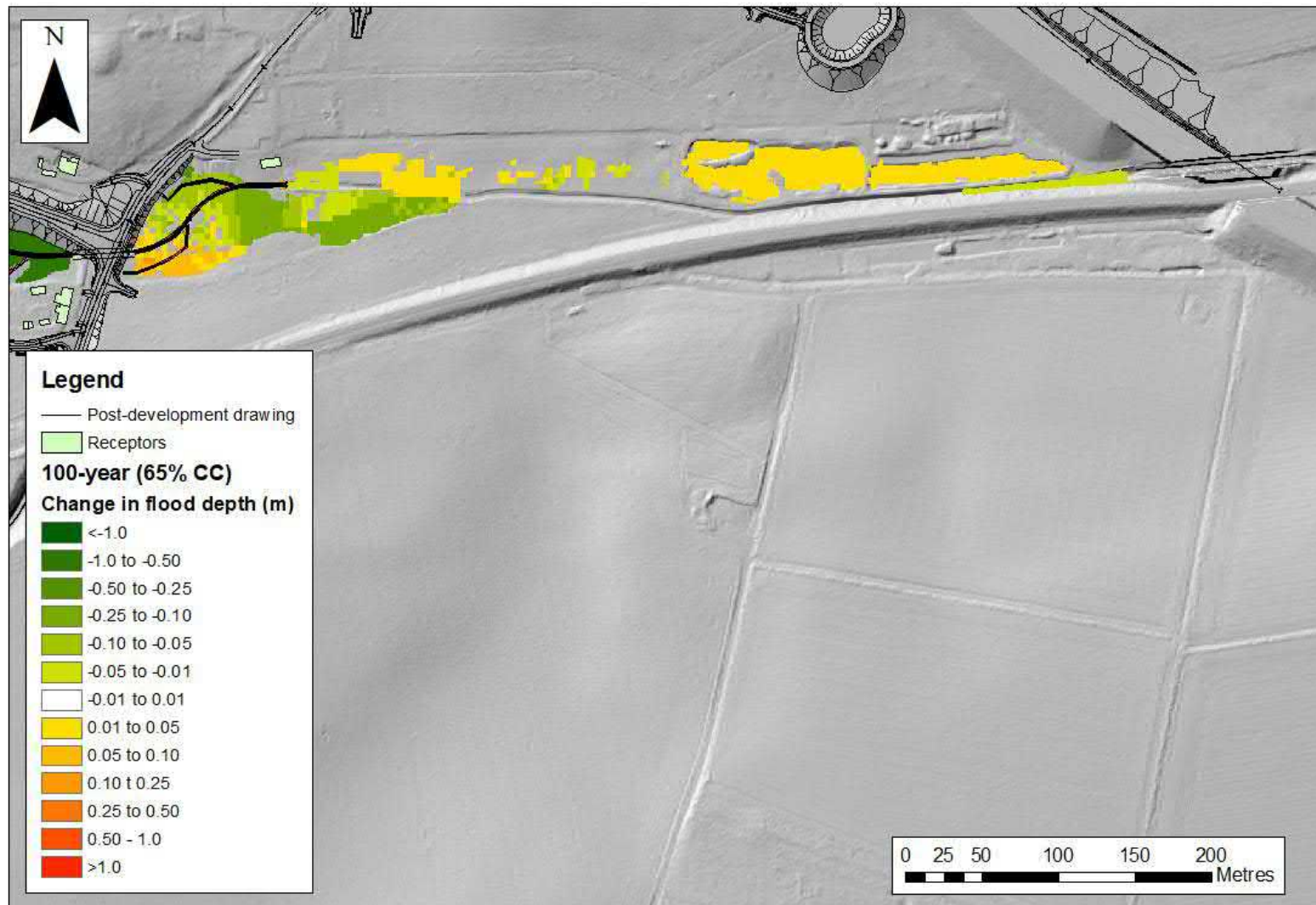
Figure C-8: Flood depth difference between Cantley Lane South and A47 (100-year plus 65% event)
