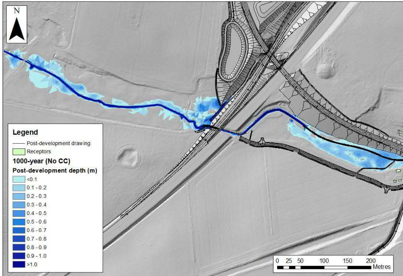
Figure C.5 : Maximum post development flood depths between upstream boundary and Cantley Lane South (1000-year event with no climate change)
