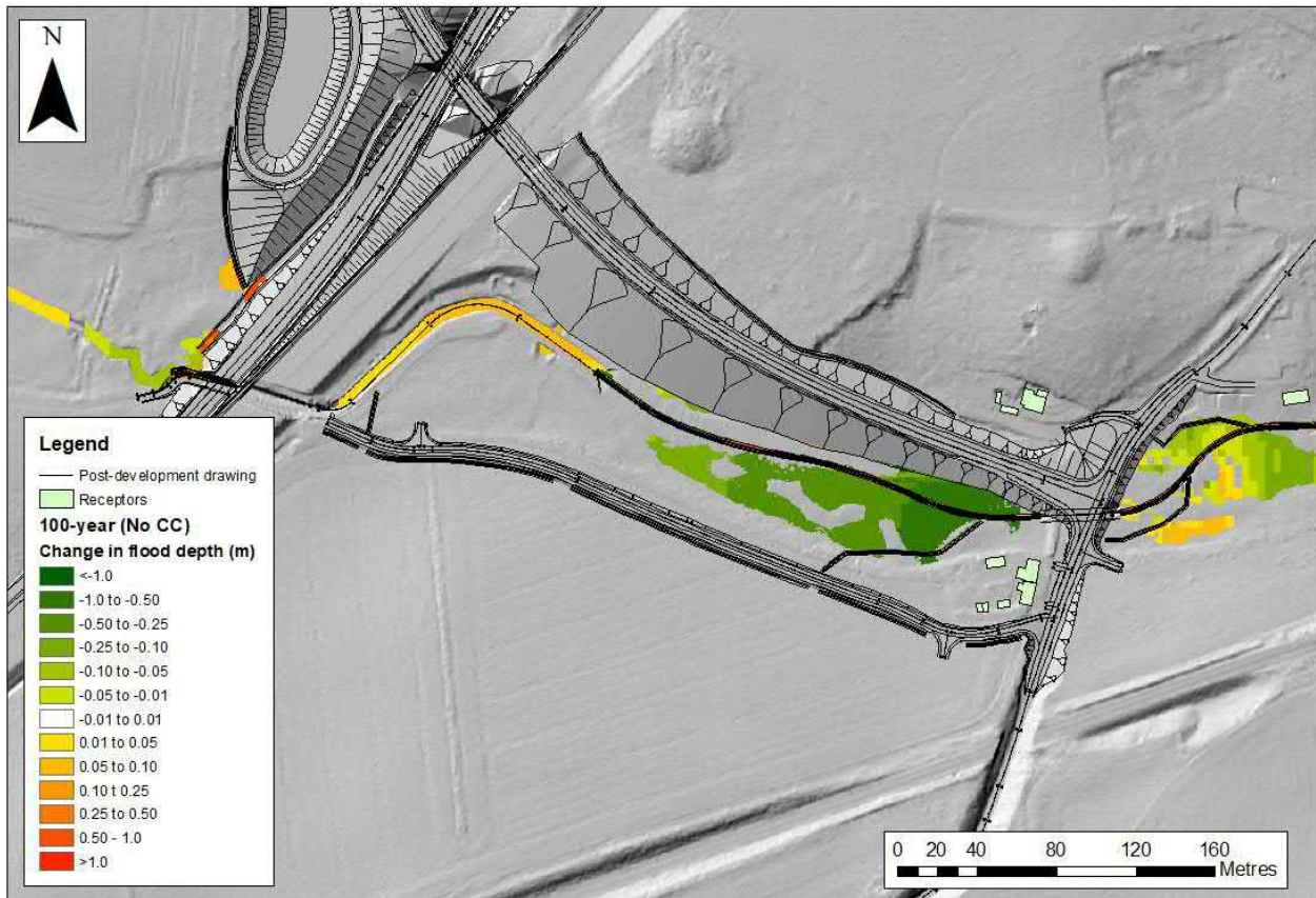
Figure 8-1: Flood depth difference for the 100-year event between the baseline and post-development model of the realigned Cantley Stream
