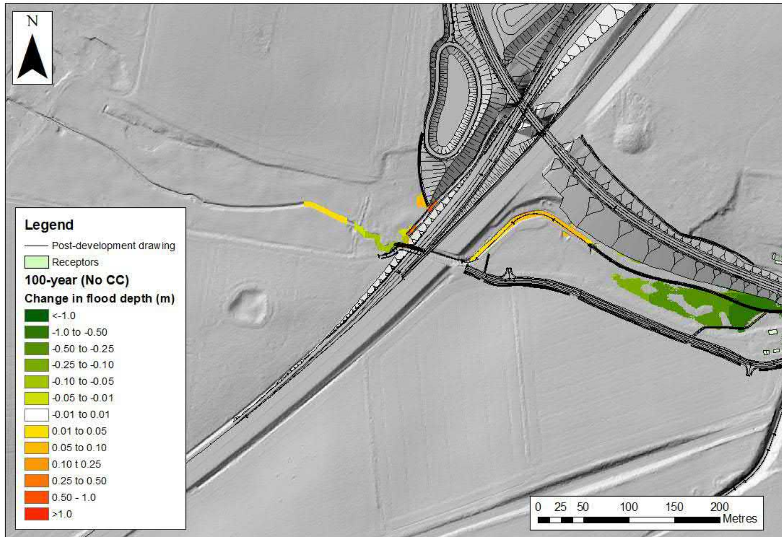
Figure C-1: Flood depth difference between upstream boundary and Cantley Lane South (100-year event)
