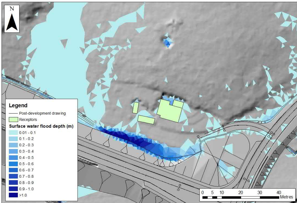
Figure 8-7: Extent of surface water flooding as a result of the drainage network
