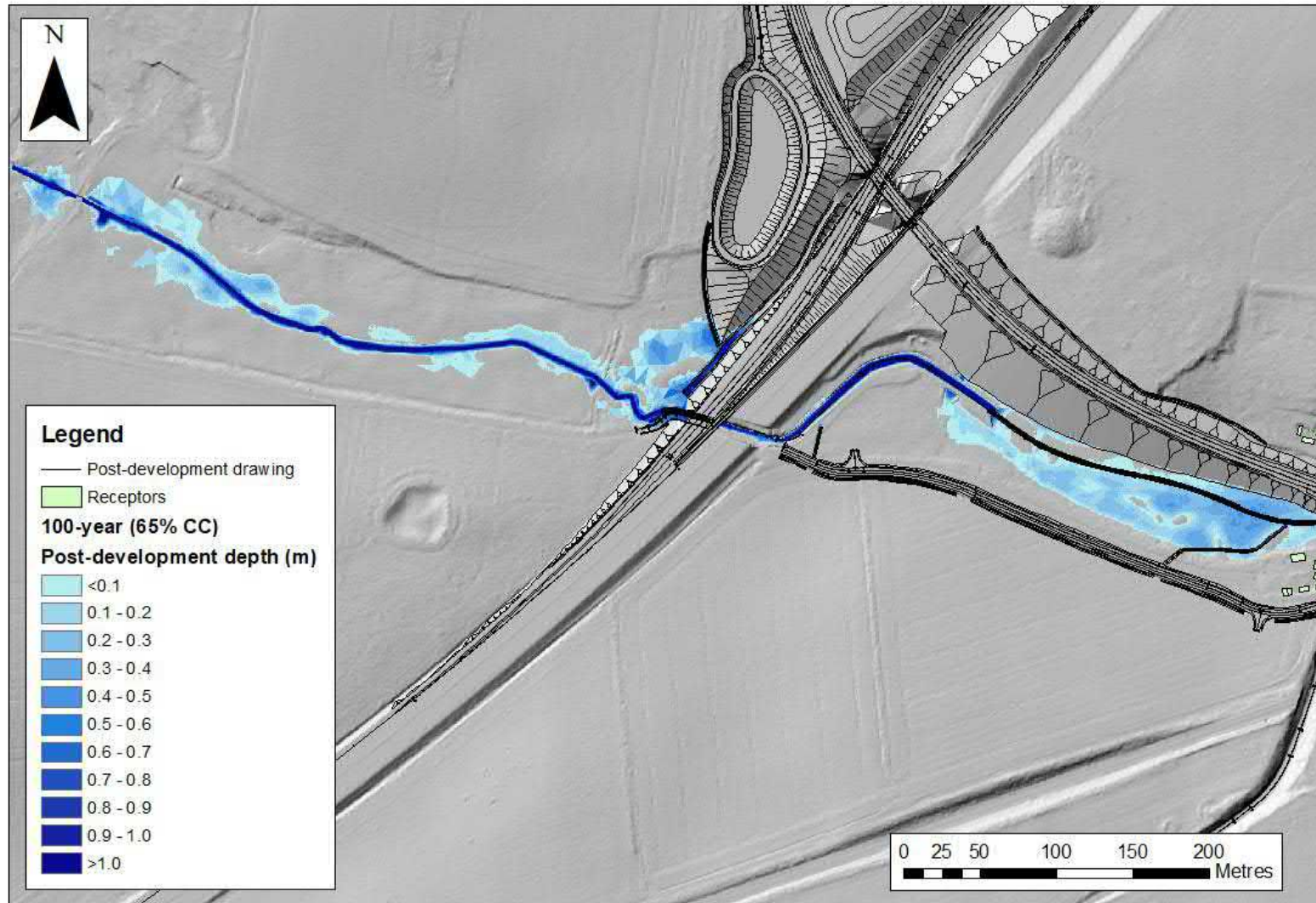
Figure C.3 : Maximum post development flood depths between upstream boundary and Cantley Lane South (100-year event with 65% climate change)
