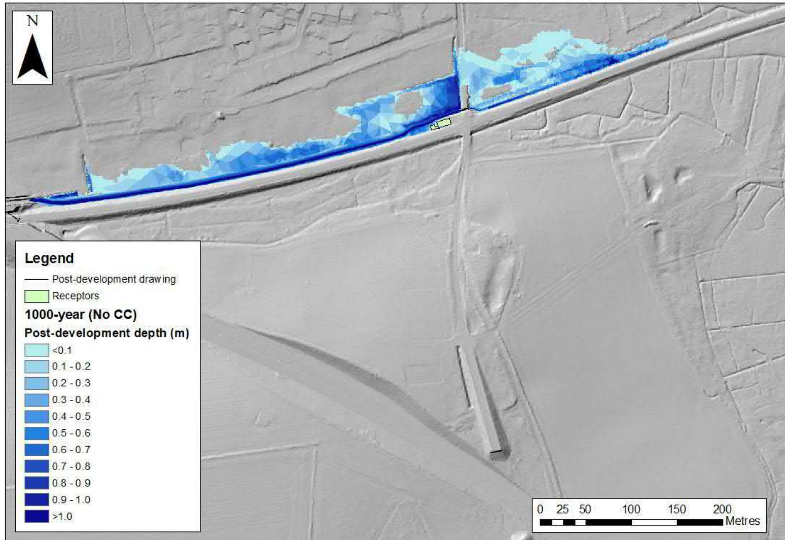
Figure C.15 : Maximum post development flood depths between the A47 and the model outfall (1000-year event with no climate change)
