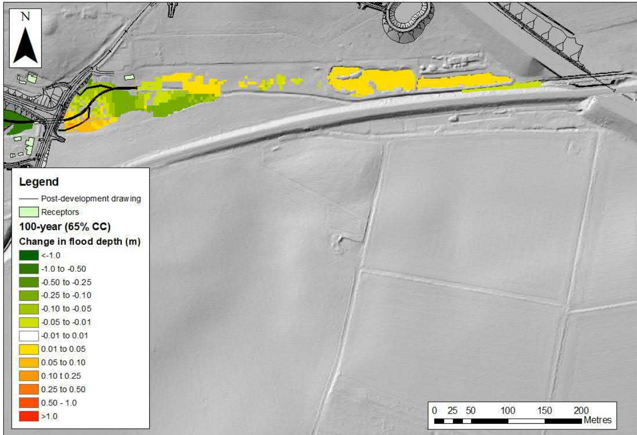
Figure 8-5: Flood depth difference for the 100-year plus 65% climate change event between the baseline and post-development model between Cantley Lane South culvert and A47
