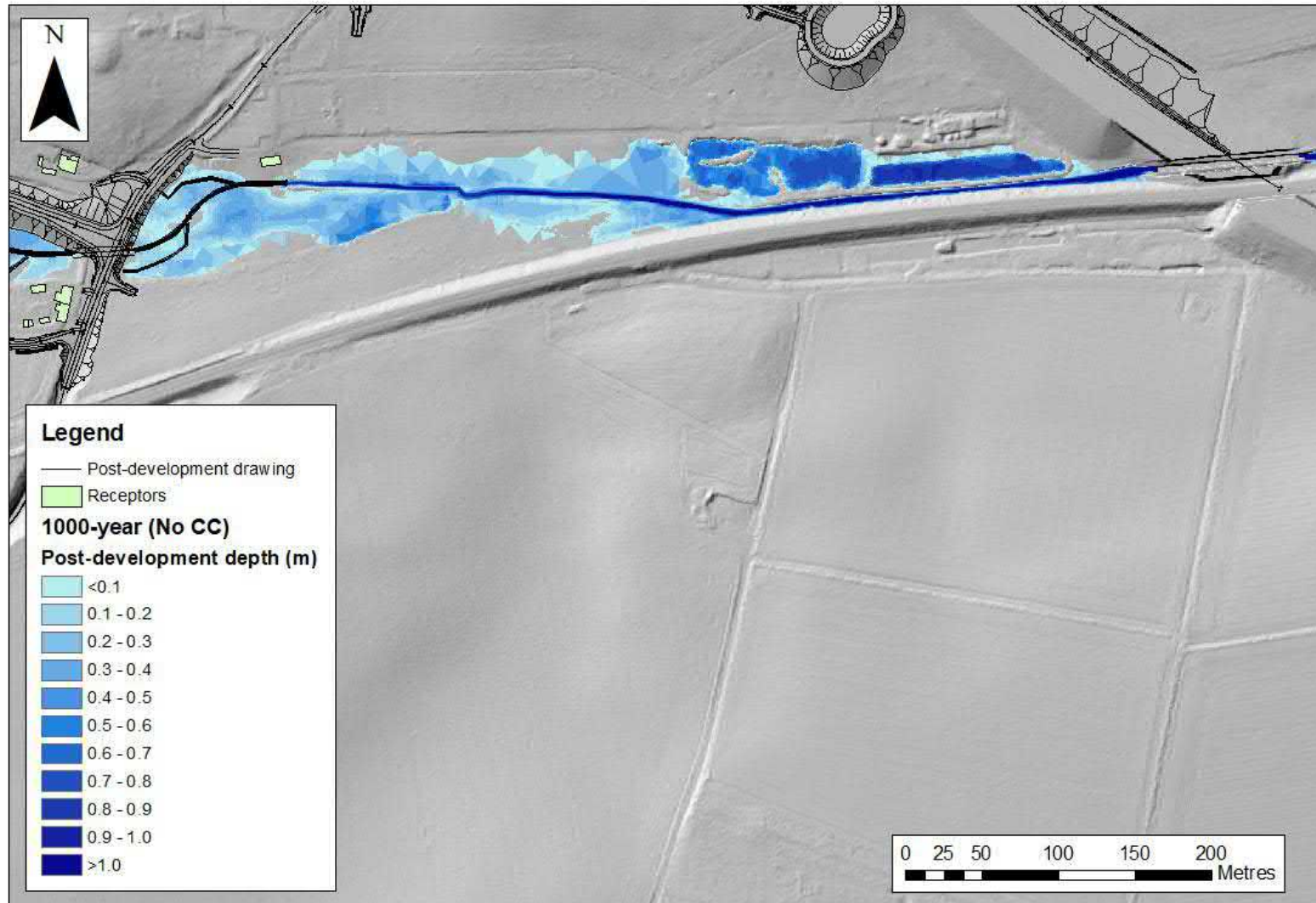
Figure C.10 : Maximum post development flood depths between Cantley Lane South and the A47 (1000-year event with no climate change)
