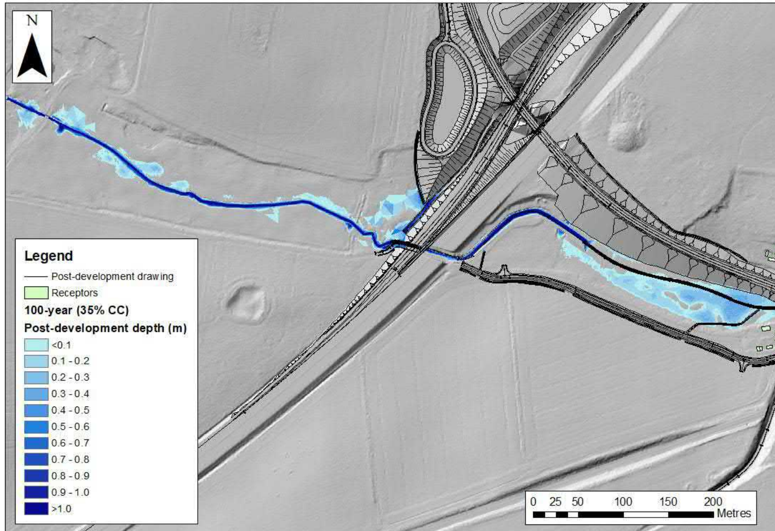
Figure C.2 : Maximum post development flood depths between upstream boundary and Cantley Lane South (100-year event with 35% climate change)
